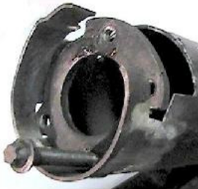
Repaired Steering Column Lower Tube
